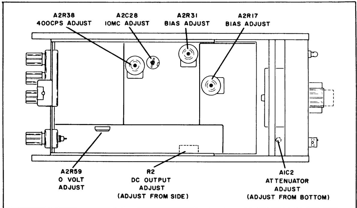
Figure 5-3. Location of Internal Adjustments
