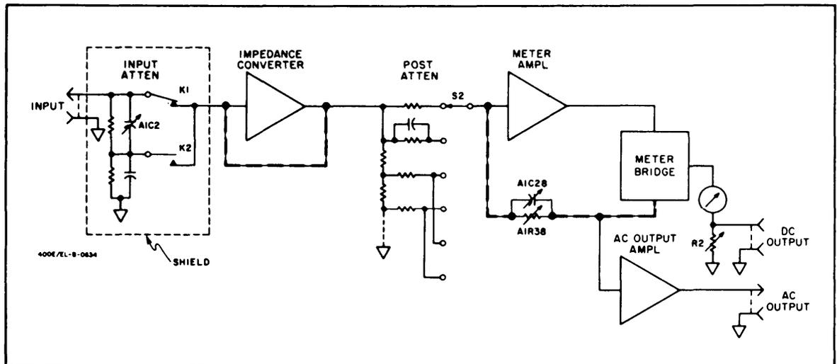
Figure 4-1. Simplified Block Diagram
