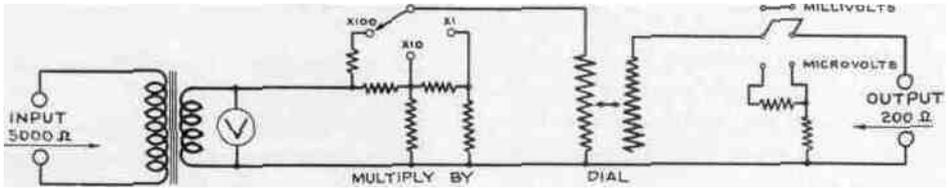
Schematic diagram of the TYPE 546-A Audio-Frequency Microvoltmeter. The open-circuit voltages shown by the calibration are obtained when the voltmeter reads 2 volts
