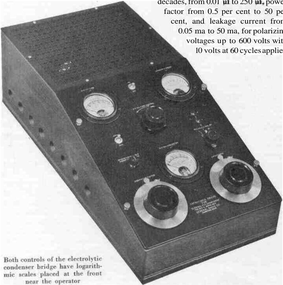
Both controls of the electrolytic condenser bridge have logarithmic scales placed at the front near the operator
