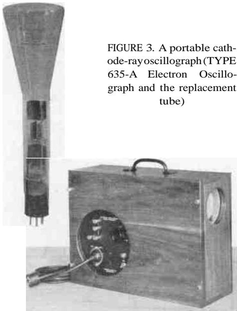
FIGURE 3. A portable cathode-ray oscillograph (TYPE 635-A Electron Oscillograph and the replacement tube)
